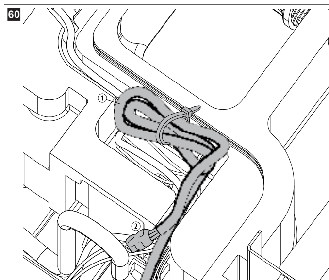
1 Bundled compressor wires 2 Taped compressor wires
