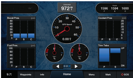
Trim tab position can be displayed on capable MFD's
